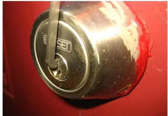
*Top of keyway/center of plug tension*
